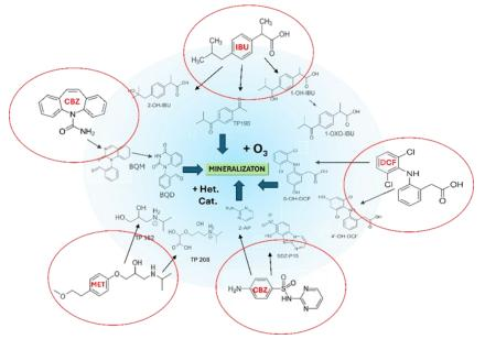
**Figure 1.** Primary transformation products identified from the ozonation of the five pharmaceuticals studied. These compounds feature a variety of reactive functional groups, including amines and quinones, which can facilitate further breakdown through additional reactions, ultimately aiding in the progression toward complete mineralization.
