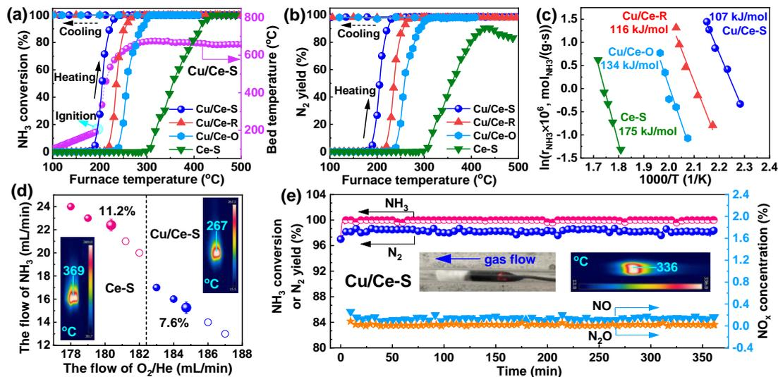
**Figure 1** NH<sub>3</sub> conversion (a), N<sub>2</sub> yield (b), Arrhenius curves (c) of catalysts, lean-combustion limits (d), and stability (e) results of Cu/Ce-S under 10% NH<sub>3</sub>+21% O<sub>2</sub>/Ar.
