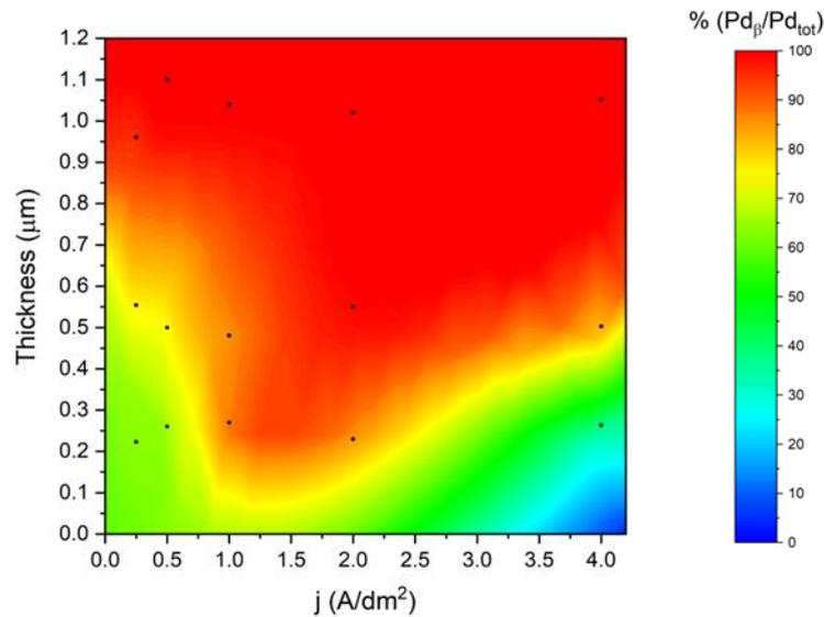
**Figure 1**  $\beta$ -PdH<sub>x</sub> percentages obtained on DC samples after 10 minutes after the end of deposition. The black dots represent the samples.
