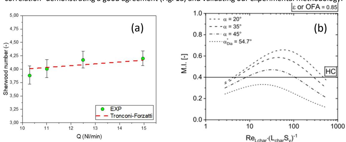
**Figure 1:** (a)  $Sh_{exp}$  (•) and  $Sh_{avg}$  T-F(---) VS operative flowrate for monolith bundle with circular channel geometry, (b) Merit Index of the modified diamond lattice as a function of  $\alpha$  at constant porosity  $\epsilon = 0.85$
